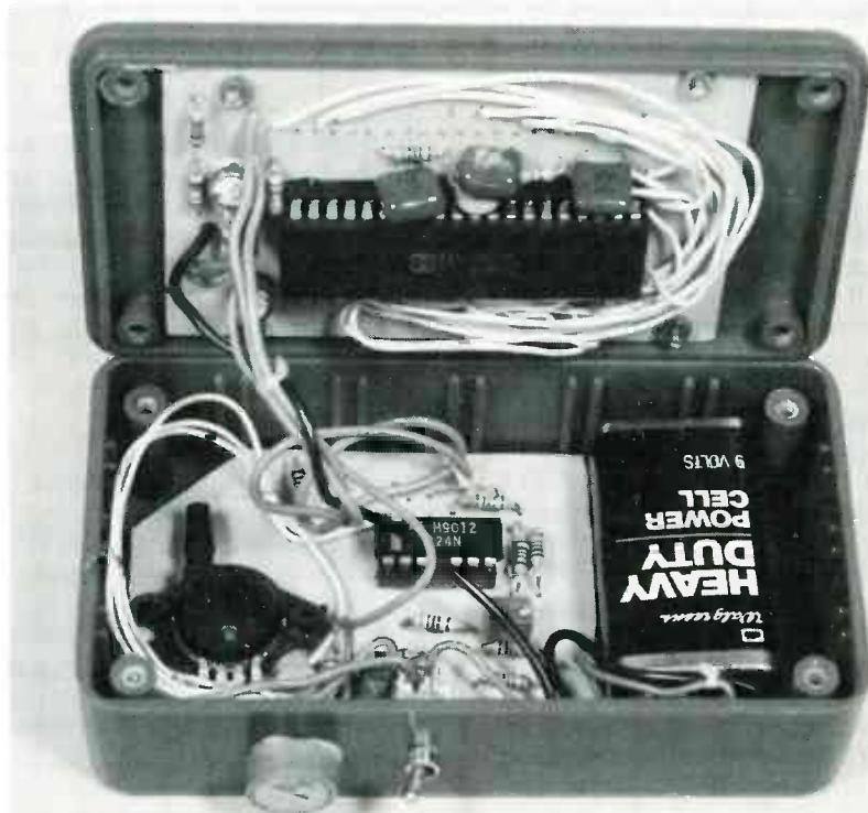
FIG. 6—HERE'S THE AUTHOR'S PROTOTYPE. Notice the four wires that connect the analog and digital boards together.
